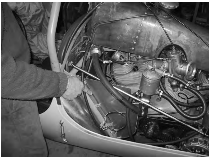
Above: Snug-fitting alloy panels deliver maximum cooling air to Garry Simkin's Cooper Vincent-engined Cooper (right at Albert Park).
