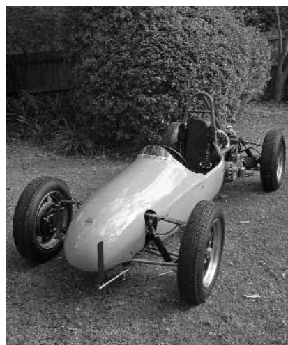
Above: The Walton-Cooper ready for Shelsley. The 'beam-breaker' at the front is mandatory for UK hillclimb timing.
